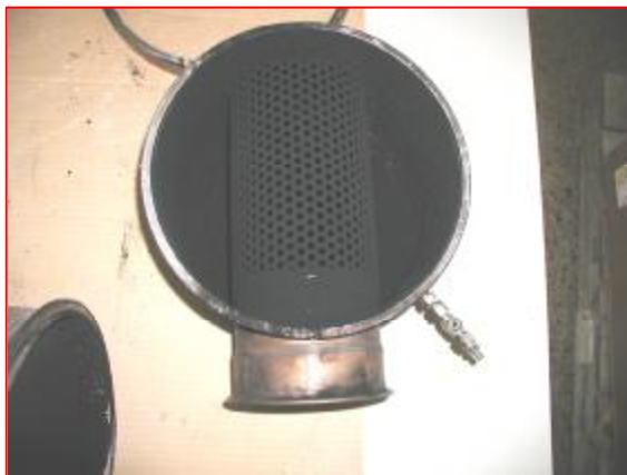
Filter Can Inlet Section
